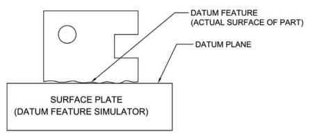
Figure 5-4 Datum feature vs. datum plane.
