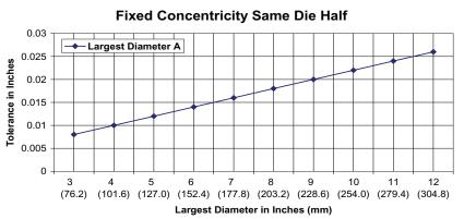
is 0.008 inches (0.20 mm). 0.002 inches (0.05 mm) is added for each of the additional 4 inches to yield a total Concentricity Tolerance of +0.016 inches (+0.40 mm) for the 7" diameter. Concentricity is defined as a feature having a common center and is usually round, circular or oval. Half the diameter is the center of the feature.
