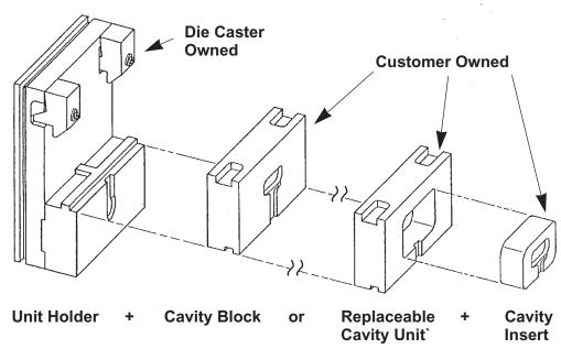
Figure 2-4 Components of a unit die illustrate each part of the assembly and the die construction option of a cavity block or a holder block with cavity insert.
