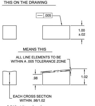
Figure 5-24 Straightness of a surface.
