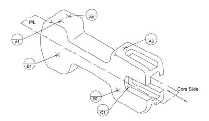
Figure 5-32 Example of a least preferred datum reference framework for a die cast part design (datums across p/l and datum on moving component). Will require qualification of all datums.
