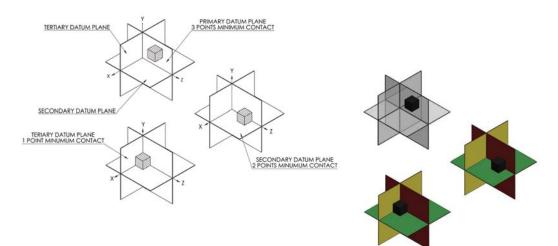
Figure 5-3 Primary, secondary, tertiary features & datum planes.
