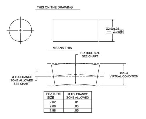
Figure 5-26 Straightness of an axis at MMC.
