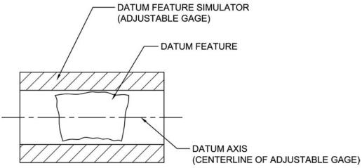
Figure 5-5 Datum feature vs. datum axis.
