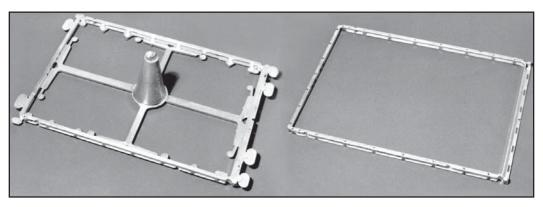
Figure 2-5 Photo on left shows untrimmed zinc die casting as it comes from the die. At right, the same casting after trimming.
