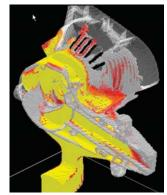
Figure 7-4: This simulation is depicting a velocity that is too slow, the metal flow is freezing before the final fill. A PQ<sup>2</sup> analysis will render a proper gate and metal flow velocity to ensure a complete fill. Simulations show very accurately the filling characteristics.
