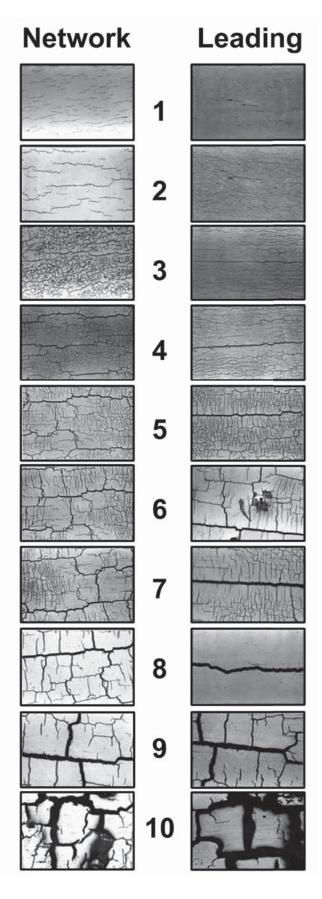
Figure 2-13 Photos of die surface crack patterns reproduced approximately 70% of actual size. The die steel heat check conditions is reflected as raised material on the surface of the casting.
