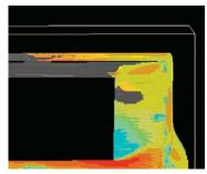
Figure 7-5b: A zinc cosmetic casting that has square corner metal flow that results in unacceptable porosity. A visual defect!
