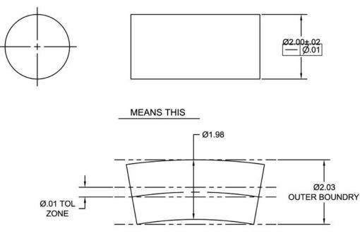
Figure 5-25 Straightness of an axis RFS.
