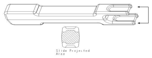
Fig. 4A-1A Proposed component with added features and design modified for cost-effective die casting production, showing orientation in the die casting die and core slide (moving die component) to cast the additional features.
