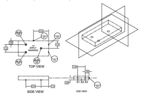
Component configuration shown as phantom lines on separate drawing
