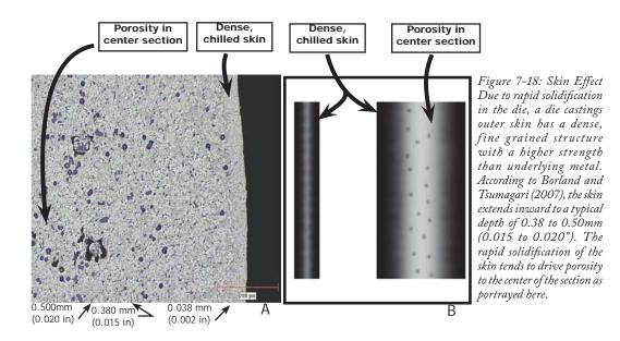
Exterior or surface porosity can be identified with the naked eye, magnification or with penetrant inspection methods.
