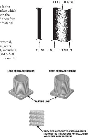
sible and very impressive when done properly, full diameter threads are generally not necessary. Wherever possible, flats to the root diameter of the thread should be allowed at the parting line. This will reduce complexity in the die and thus lower initial tooling charges and piece part costs.
