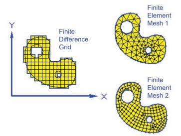
Figure 7-11 A: 2D illustration of the difference between finite difference and finite element meshes.
