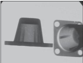
Figure 7-21B: Example radiograph of porosity that does not impact part form, fit or function. The user should be agreeable to accepting a specified amount of porosity in areas of the casting where it does not impact form, fit, or function.
