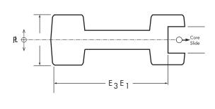
Projected Area is the area of the core head that faces the molten material. MDC Tolerance for moving die components is determined from table S-4A-3. The open area (cavity) on the end view of the part in figure 4A-1A at the beginning of this section shows the projected area. Projected Area Tolerance plus Linear Tolerance provide MDC Standard Tolerance for the volume of the part. Note that the tolerances in the table apply to a single casting regardless of the number of cavities.
