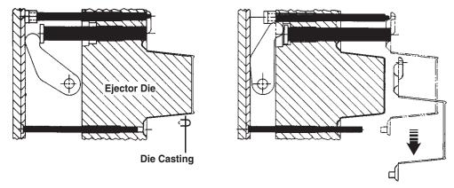
Figure 2-9 Ejector pins, shown in black, are recessed as the metal fills the die cavity (above left); then actuate sequentially to release the casting from the die (above, right).
