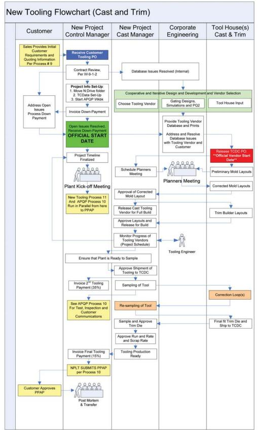
Figure 7-24: Example New Tooling processes flow chart.
