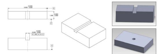
Figure 5-13 Positional tolerance for keyway.
