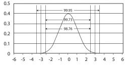
Figure 7-16: CPK indicates a normal distribution that allows within the distribution the maximum allowance of plus/minus tolerance that yields the greatest number of good parts in production. The higher the CPK number the more repeatable and accurate the process is.
