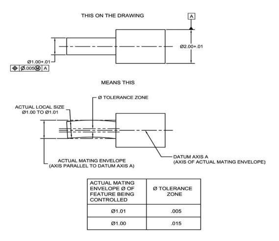
Figure 5-9 Position control with MMC.
