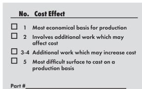
This Finishing Checklist provides a convenient method for assuring that important factors involved in the surface finishing of cast parts are evaluated and clearly communicated between the purchaser and the caster.
