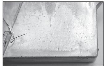
Figure 2-12 Washout as seen on a casting.
