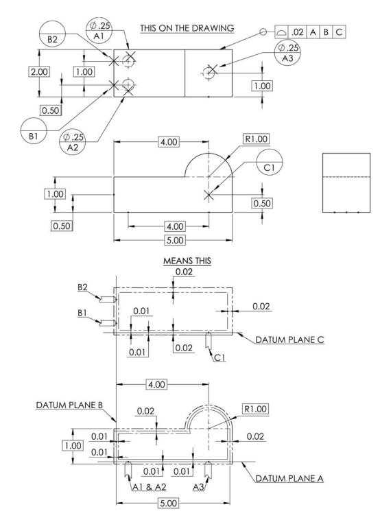
Figure 5-18 Profile control – all around entire part with targets.
