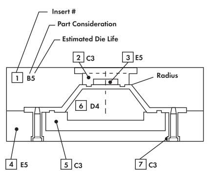
Last is to develop the matrix for communication of tool steel replacement needs and to develop history on each insert. (The information shown in this example represents only what can be done. The actual information to be included should be determined by the customer and the die caster). Two examples of this type of matrix are shown, at the start of a new project and the other as it may appear after the first year of production.
