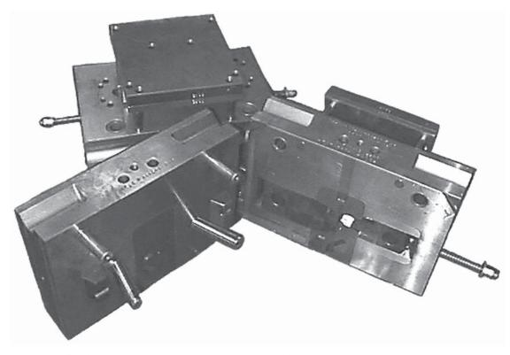
Figure 2–2 A "unit" die casting die, like the one above, allows use of replaceable cavities in standardized main die frames for lower die costs.
