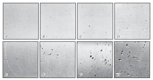
Figure 7-19: Various degrees of porosity exposed after machining.
