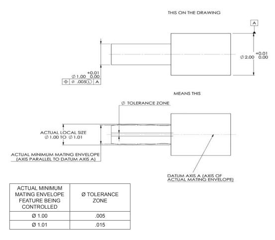
Figure 5-10 Position control with LHC.
