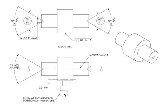
Figure 5-19 Circular runout with targets.
