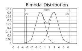
Figure 7-15: Cp can be applied to a bimodal distribution that allows for migration from one side of the tolerance range to the other. The higher the Cp number the more repeatable the process is.
