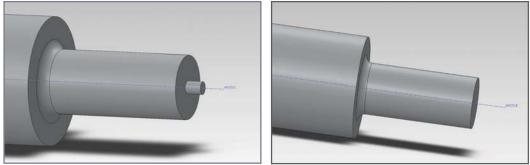
Figure 5-14 Concentricity tolerancing.
