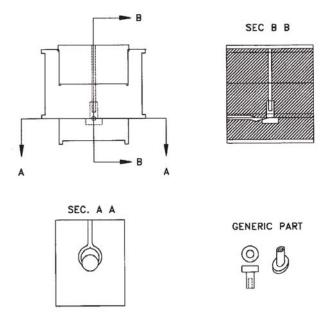
Figure 4B-5 Typical gating system in a miniature die casting die.
