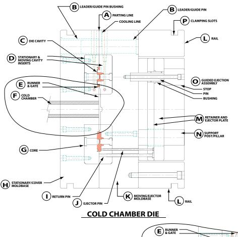
Figure 2-1 Shown above is a multiple-cavity cold chamber die casting die. With this process the metal enters the die runners, gates and cavity through the cold chamber. The Sprue replaces the cold chamber in the hot chamber process which is used for zinc and smaller magnesium components.
