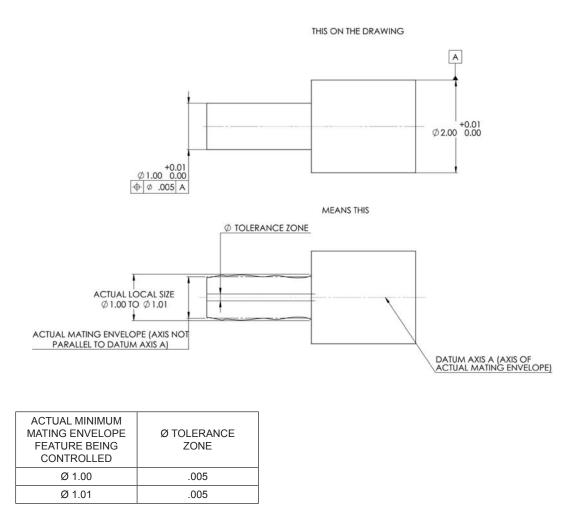
Figure 5-11 Position control with RFS.
