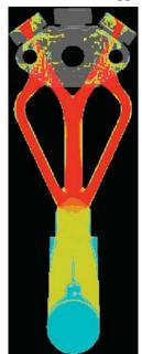
Figure 7-1: This is an example of the overflows filling first instead of being the last place to fill. An initial fast simulation will detect such undesirable characteristics.
