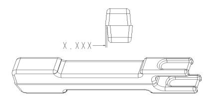
Table S-4A-6: Parting Line Shift Tolerance (Excluding unit dies)
