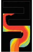
Figure 7-5a: Square corners in a runner or casting result in porosity. pockets.
