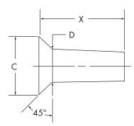
available on the thread. The fitting should not bottom out in the hole. Standard taper is normally <sup>3</sup>/<sub>4</sub> inches per foot. However, taper for special applications is determined by required strength formerly discussed in Cored Holes for Formed Threads.
