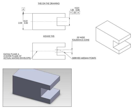
Figure 5-15 Symmetry tolerancing.
