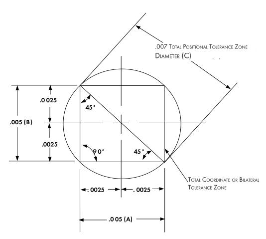
Figure 5-33 Conversion of positional (cylindrical) tolerance zones to/from coordinate tolerance zones.
