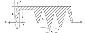
Drawing defines draft dimensions for interior and exterior surfaces and total draft for holes (draft is exaggerated for illustration). NADCA
