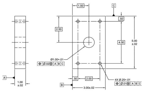
Figure 5-12 Positional tolerancing of holes.
